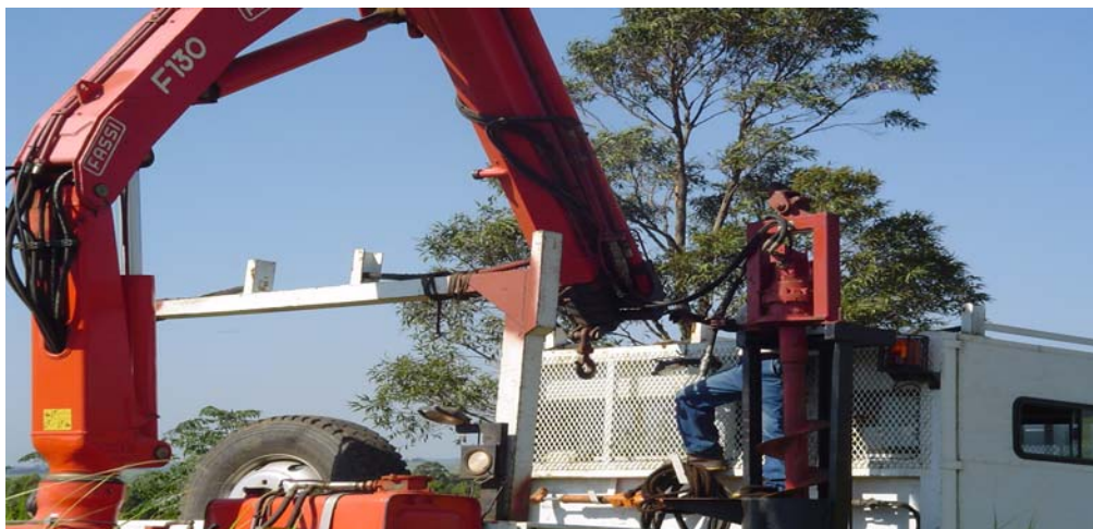
Figure 8: Auger hydraulic pipes being stowed
