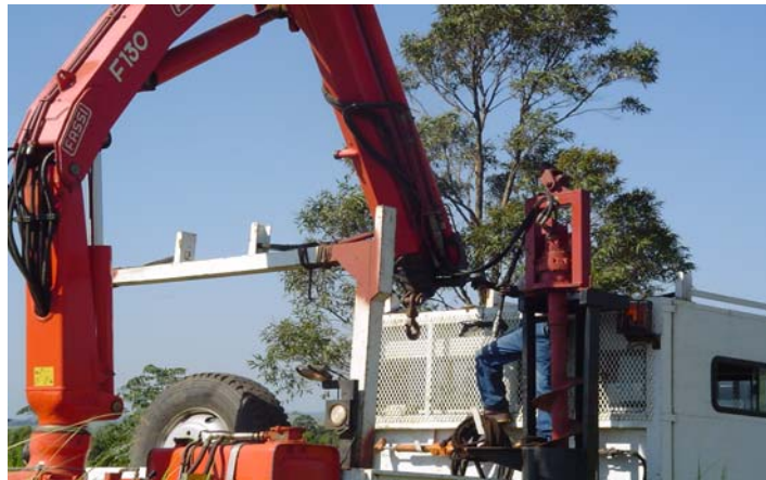
Figure 4: Auger hydraulic pipes being connected
