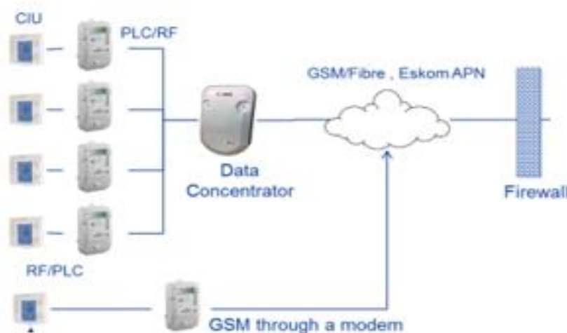
Figure 1: Simplified Smart Meter Architecture
