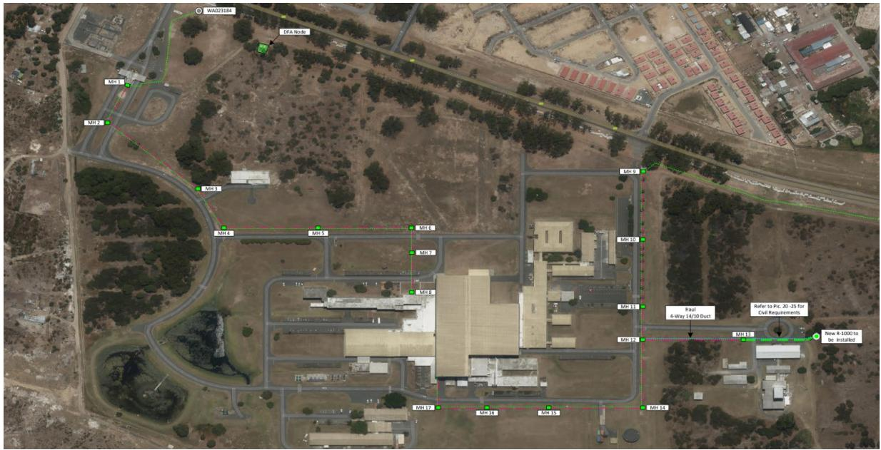
Figure 1: iThemba LABS Existing Fibre Infrastructure
