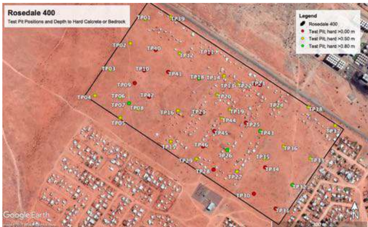
Figure 5. Site layout, test pit positions and depth to hard calcrete or bedrock (© GoogleEarth).
