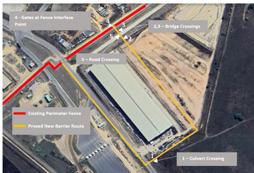
Figure 3: Proposed Routing for Perimeter Security Infrastructure
