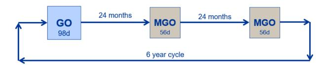
The life expectancy of each Electrostatic Precipitator (ESP) at Kriel Power Station is at least 25 years from the midlife upgrade or refurbishment. Components such as pedestal bearings, tumbling hammers, v-pads, anvils, inlet, outlet screens and turning vanes as well as refurbished components are to last at least 2 years of operation, which is until the next mini outage (MGO).
