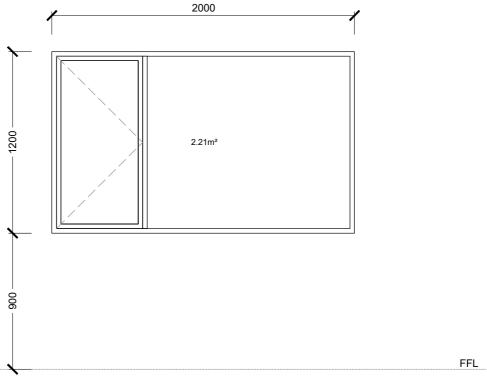
Type. A Crealco Swift 38 or eq. approved side hung aluminium casement window, per layout. Casement sash 700 x 1500mm max size.
