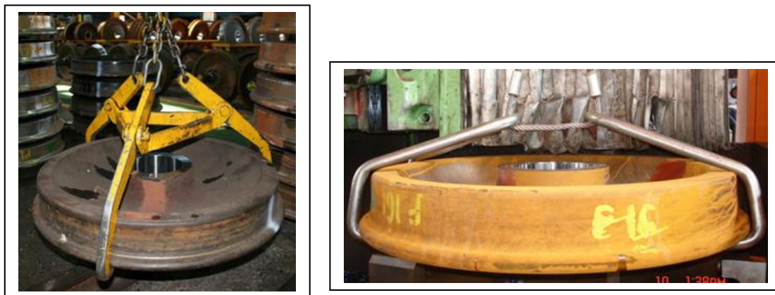
Figure 7: Wheel centre lifting devices – horizontal clamping.
