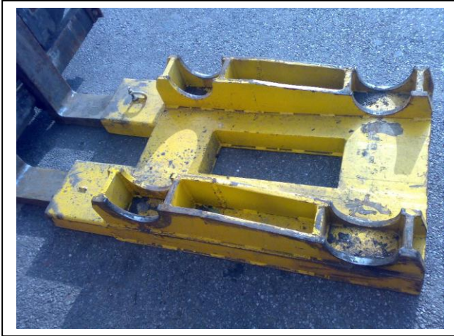
Figure 4: Forklift wheelset transportation rack as per drawing TWK12229 for a 3 ton forklift and TWK19377 for a 4 ton+ forklift.
