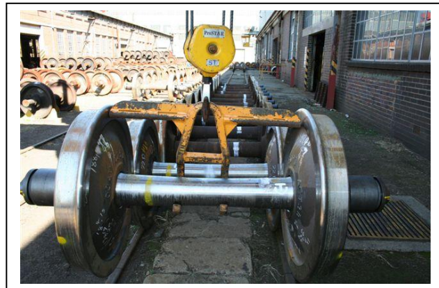
Figure 3: Wheelset lifting device as per drawing.
