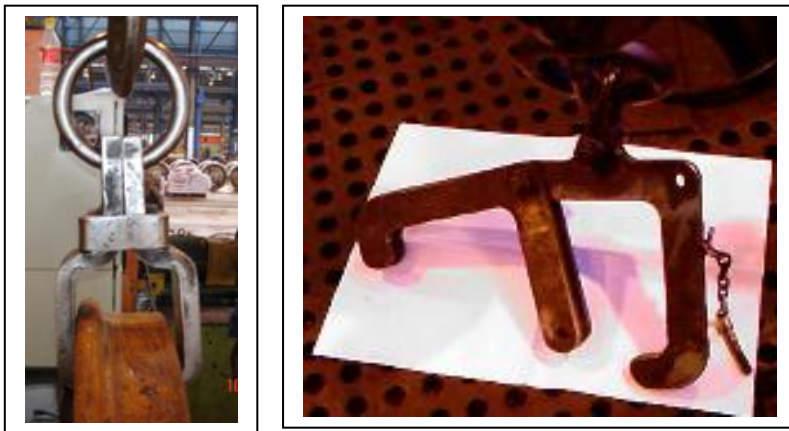
Figure 6: Wheel centre lifting devices – vertical clamping.
