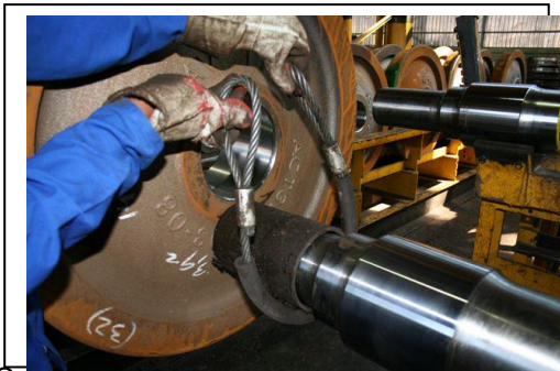
Cable covered with rubber lining to prevent journal damage, or dolly sleeve must be placed over the journal before lifting with a bare cable.
