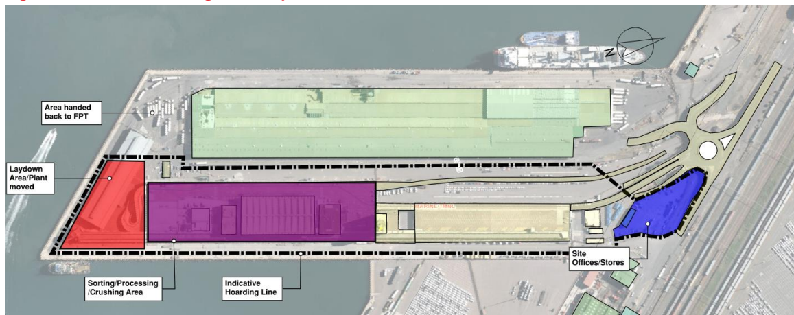
Figure 7: Phase 1a hoarding and site plan post demolition of N-shed, Spiral ram, and passenger tunnel
