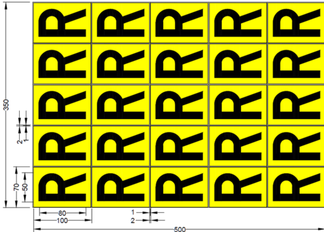
Figure 17 – Pole label "R"
