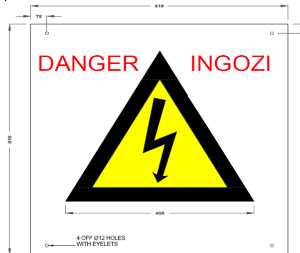
Figure 44 – Screen printed chromadek substation danger plate sign
