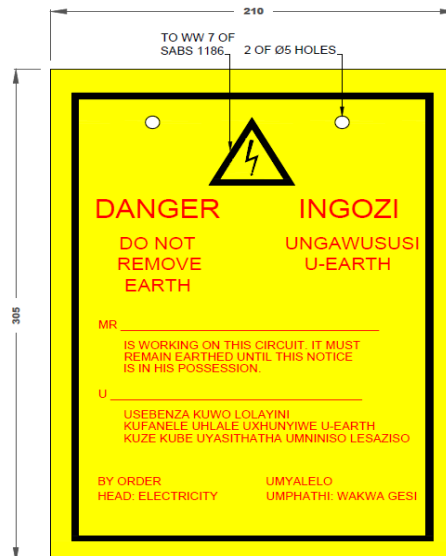
Figure 29 – Hardboard "Danger do not remove earth" sign
