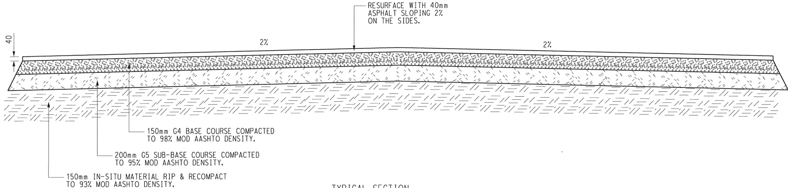
TYPICAL SECTION THROUGH RE-SURFACED ASPHALT
