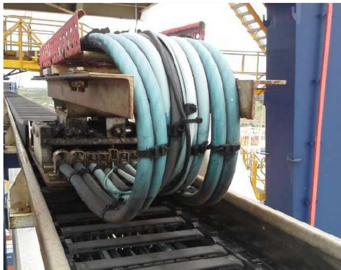
Figure 3: Floating head to be refurbished
