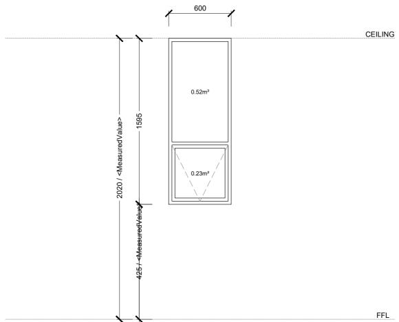
Type. P Crealco Swift 38 or eq. approved top hung aluminium casement window, per layout. Casement sash 1500 x 1200mm max capacity
