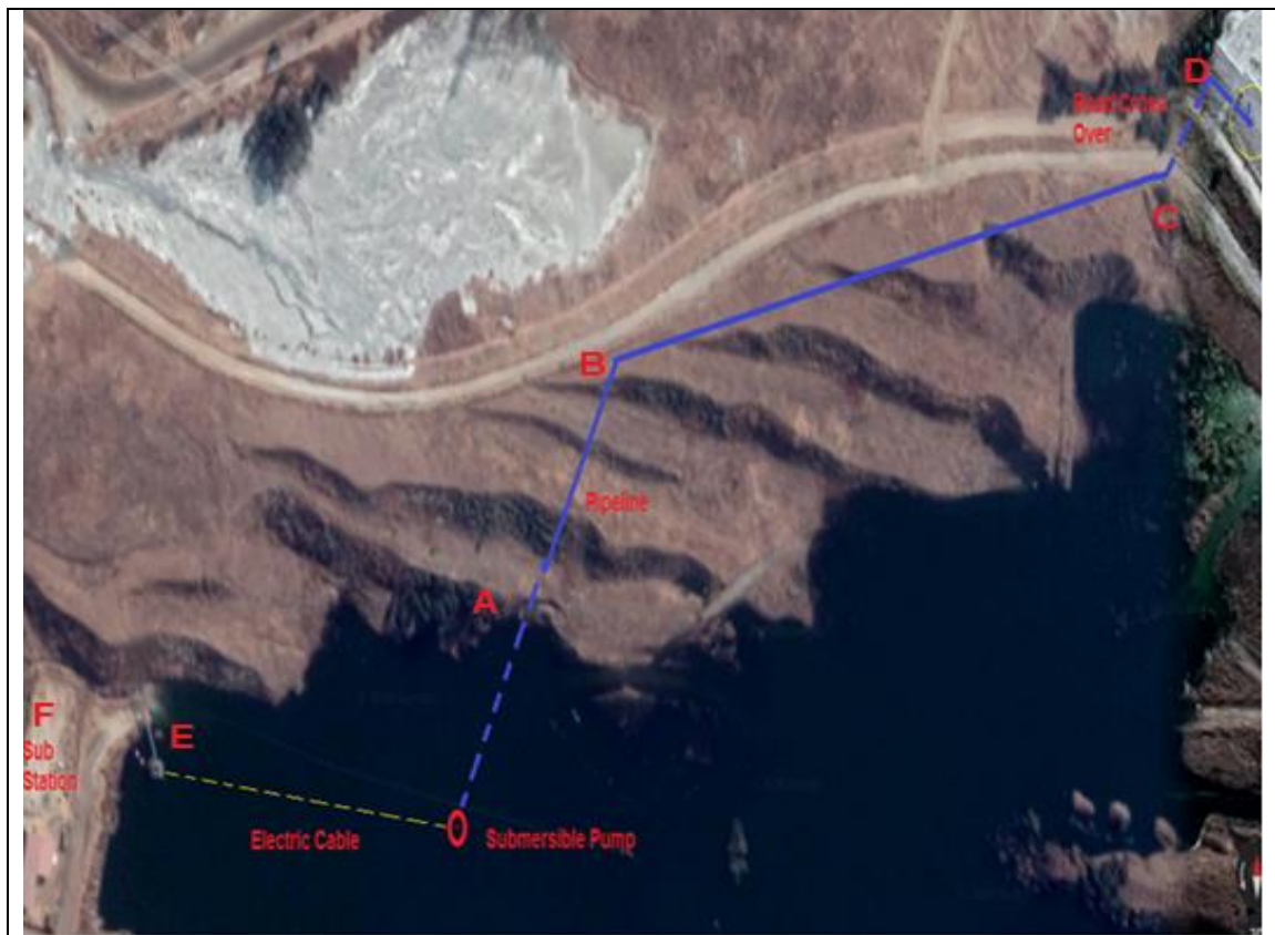
Figure 1: Site Arrangement Pipe line layout Proposal
