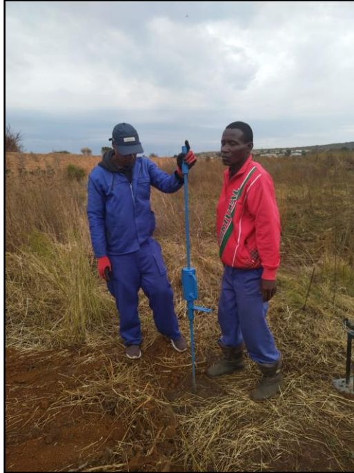
Figure 4: DCP testing conducted on site at TP08.
