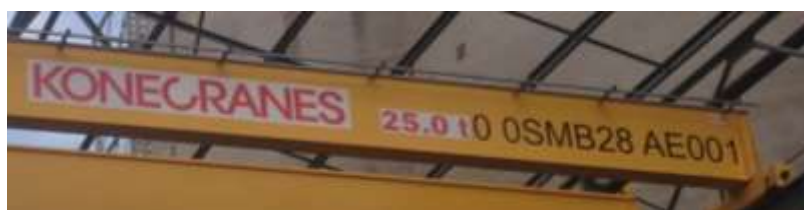
Figure 40: KKS code placing on Cranes & Crawl beams
