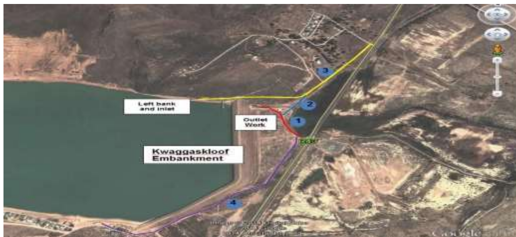
Figure 3: Plan view of Kwaggaskloof embankment (Google Earth, 2013)
