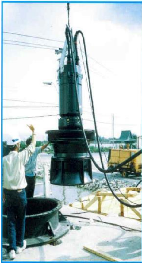
VERTICAL SUSPENDED COLUMN WITH VERTICAL DISCHARGE
