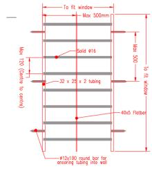
All steel joint to be welded If width of window exceed 1m, install 40x5 flat bar every 500mm
