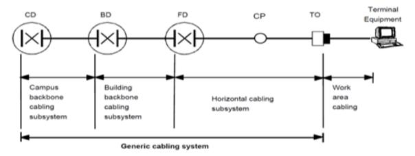
\*Consolidation points: Shall only contain passive connecting hardware and shall not be used for cross-connections. A consolidation point should be located in accessible locations [but not to the public]. The consolidation point shall be located so that there is at least 15 m from it to the outlet.
