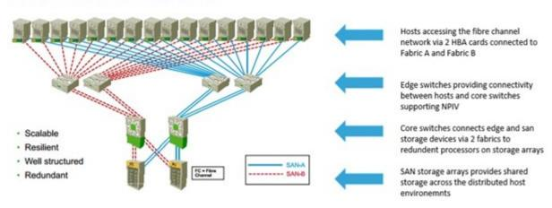
The core switches, located in all main data centres, utilizes 48 ports with 4 additional QSFP port or 96 port with 8 additional QSFP port switches capable of 32Gbps speeds with either single mode or multi model SFP's and cabling. Inter Switch Links (ISL) connectivity between each switch is provided via 4 single mode fibre links configured as a single trunk.
