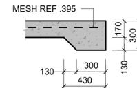
**SLAB EDGE THICKENING DETAIL**
