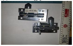
13.16 M00000226 - bolt, barrel; finish polished, dimensions wide 25 x length 75 mm, material, brass, special features brass shoot diameter 8 mm; p/n: b517 boustreds art 205, solid/esco; used on cabinet door, etc, part number or equal, solid, drawn, heavy pattern to quoted
