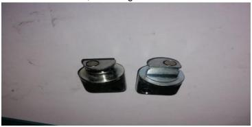
13.32 M00032192 - key; type controller, material conforms to drawing: CEE - THT - 147 / latest; equipment used on motor coach 5m2a, push button switch box
