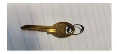
12.42 M00001244 - key, lock: type: pad: mfr: viro p/n: m024502/a8372: item to be die-stamped users description see item M00053918 for lock, equipment used on padlock no 2049 configuration sig
