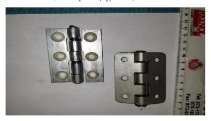
13.20 M00010918 - hinge, butt; length 2-1/2 inch, finish satin chrome, features steel pin, 3 screw holes per leaf, open, material brass, type butt, width 2-1/4 in;
