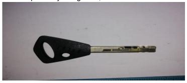
13.31 M00101289 - key; type driver control key, special features used on 10m5 motor coach, with magnetic shaft
