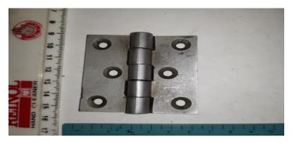
13.21 M00033287 - hinge, butt; length 3 inch, finish satin chrome, features brass pin, 3 screw holes per leaf, material brass, butt width 2 inch; users description end door; used on surburban coach 5m2a mainline coach gd-1 main
