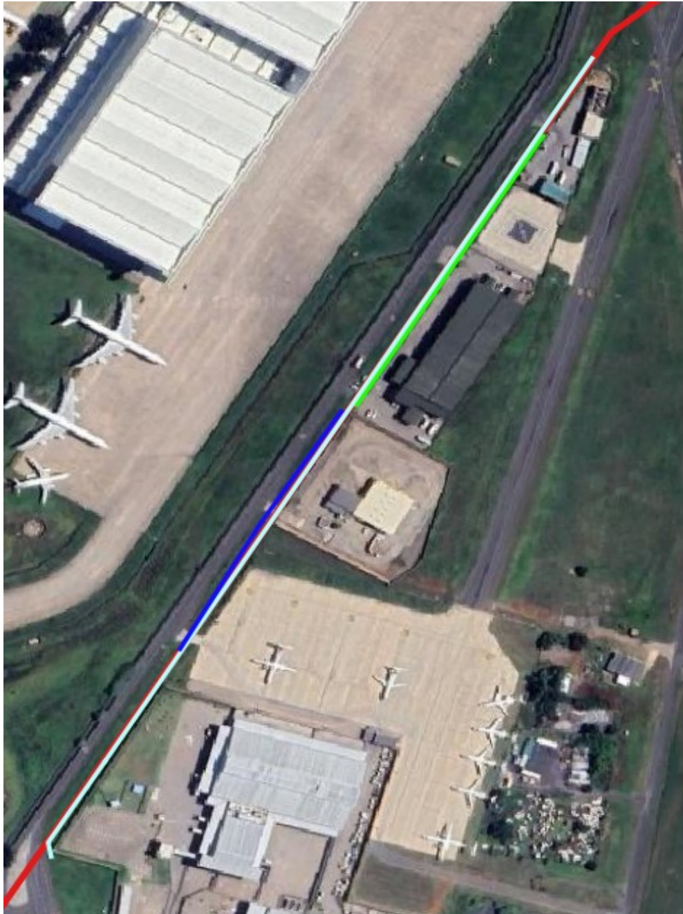
Figure 11: Red = Original 20 Inch line; Green = Buried 11 kVA line, Blue = Buried 1 kVA line, Cyan = Buried Optical Fibre line.
