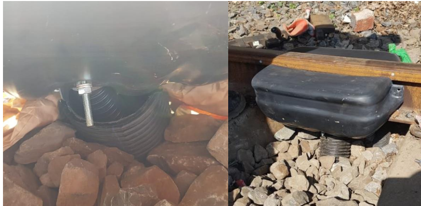
Photo 13: Axle Counter Equipment: 2 types of Kevlar cover Head protection
