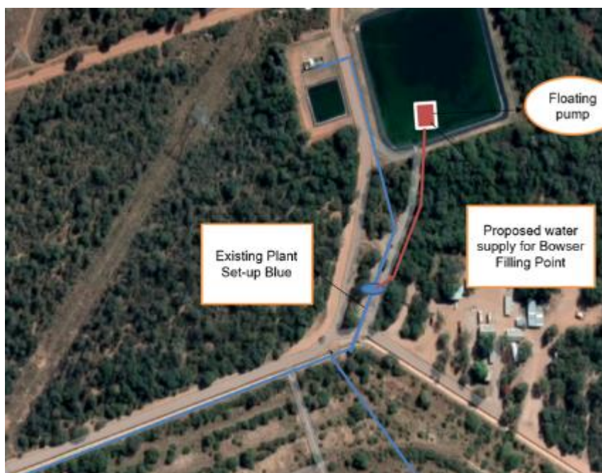
Figure 2: Irrigation system with Bowser filling system and the proposed pumping system layout.
