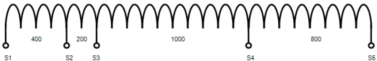
Figure 5: Tapping Arrangements for Multi-ratio 1/2400
