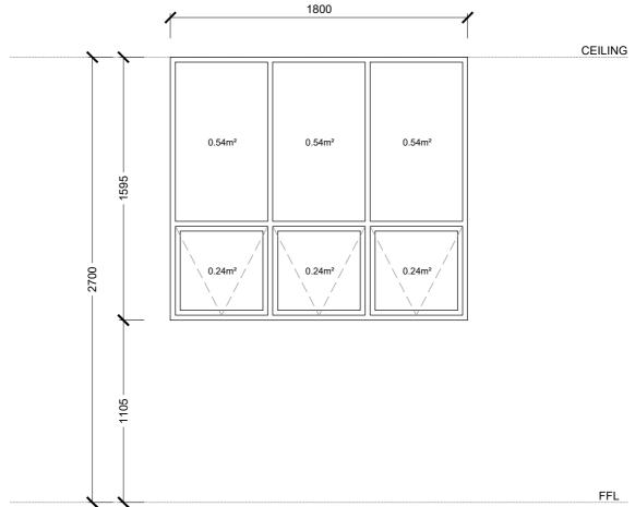
Type, M Crealco Swift 38 or eq. approved top hung aluminium casement window, per layout. Casement sash 1500 x 1200mm max capacity
