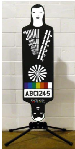
Figure D.1: Rotakin Test Target
