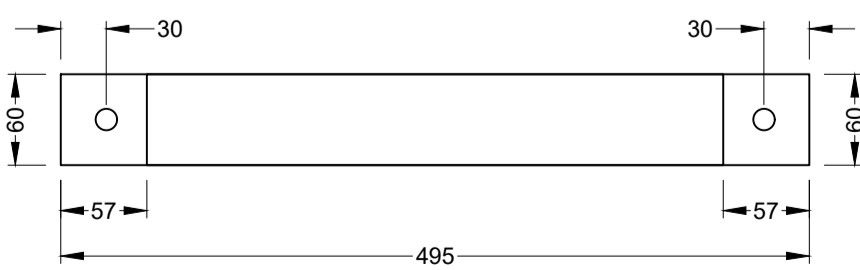
200mmØ PIPE BRACKET CUT PROFILE Scale 1 : 5
