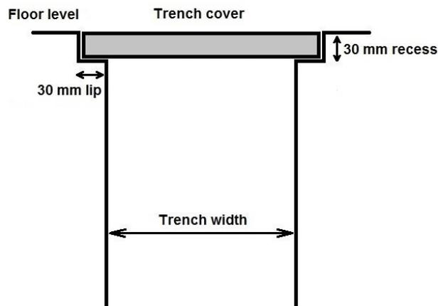
**Figure 2 – Typical trench detail for item 3**
