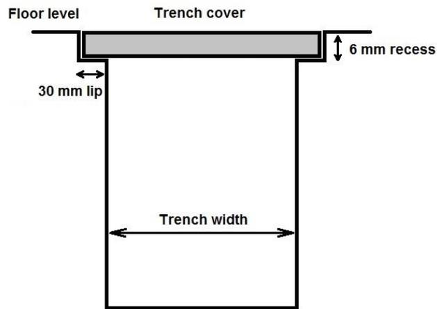
**Figure 1 – Typical trench detail for items 1 and 2**
