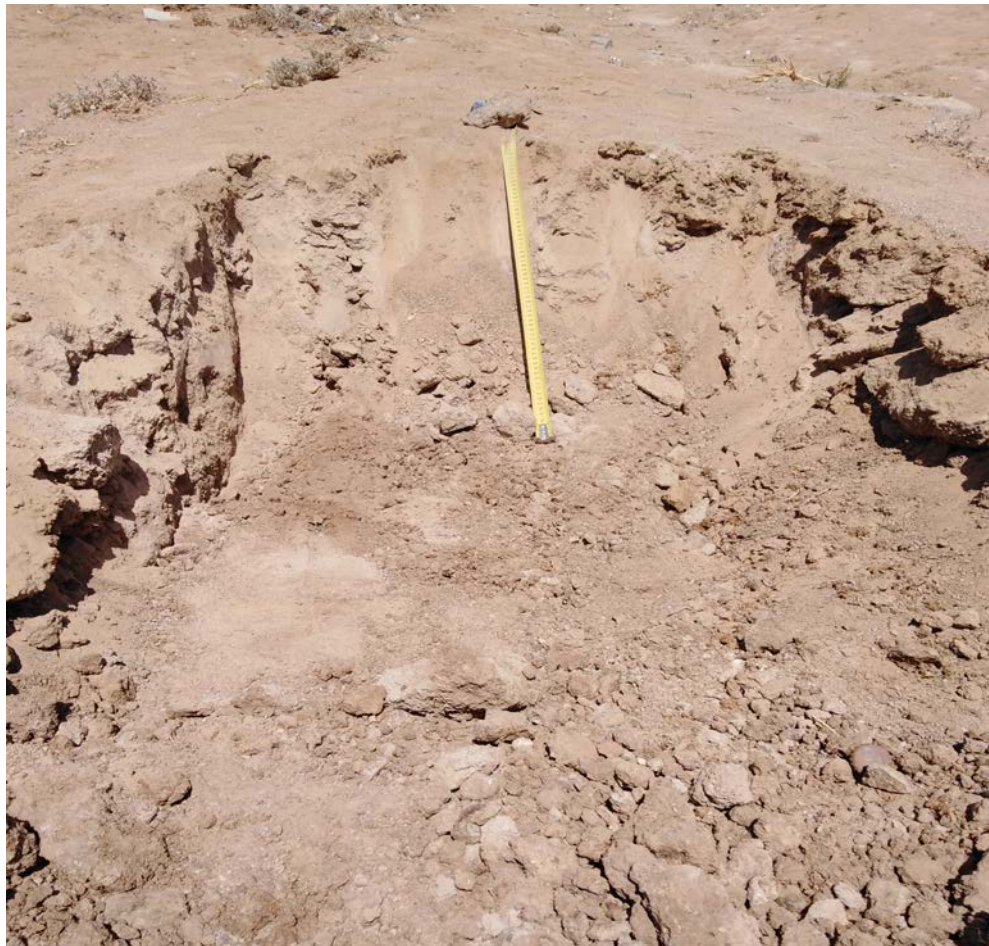
Figure 6: Test pit showing the transported horizon
