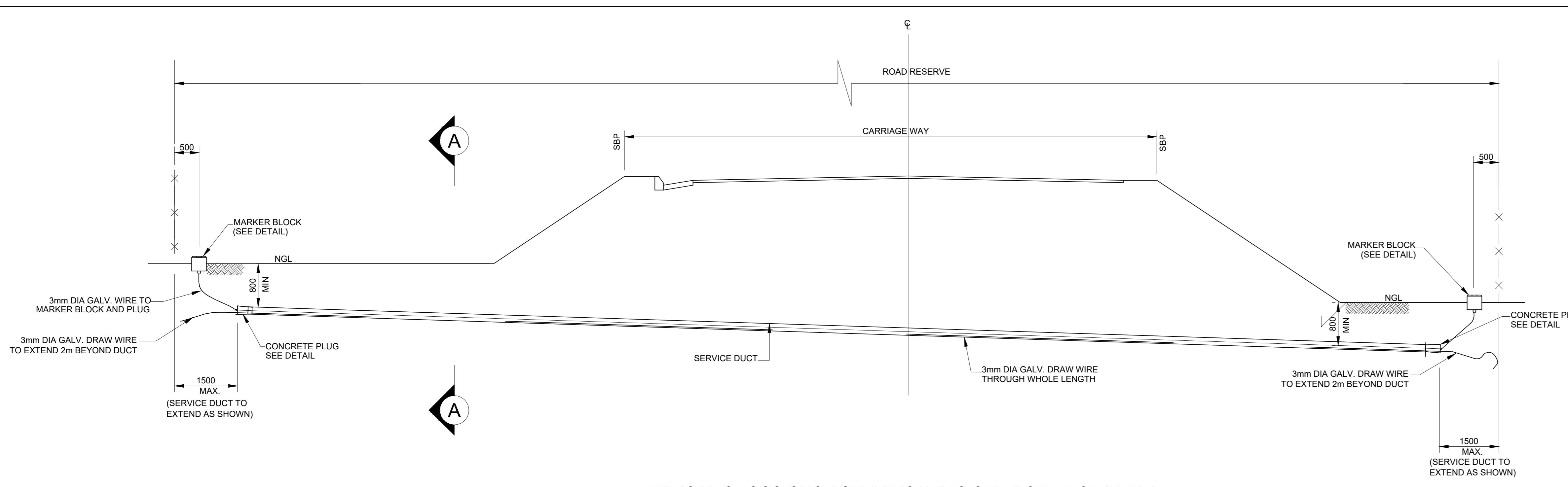
TYPICAL CROSS-SECTION INDICATING SERVICE DUCT IN FILL
