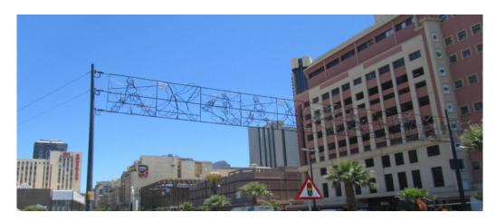
Set-pieces installed on catenary wire. Set-piece size is 2 x 2.1m. Adderley Str
