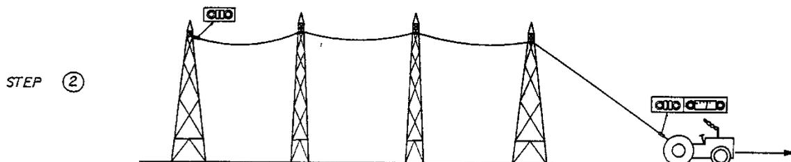
**STEP 3: SLACKING OF CONDUCTOR**
