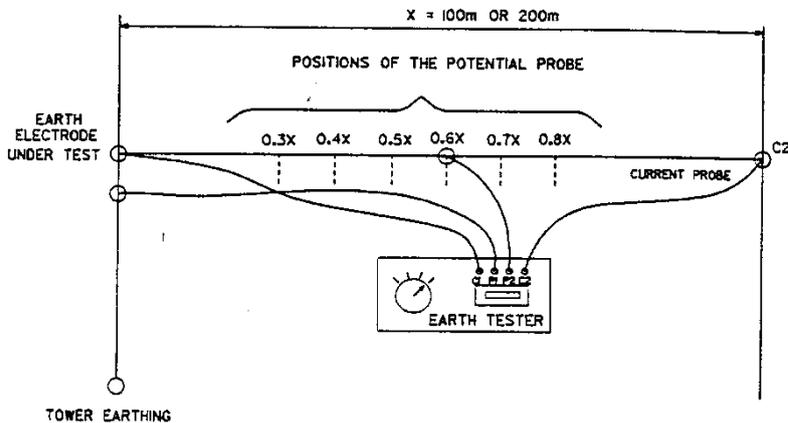
**FIGURE 1: CONNECTIONS FOR EARTH ELECTRODES RESISTANCE MEASUREMENT - 61.8% METHOD**
