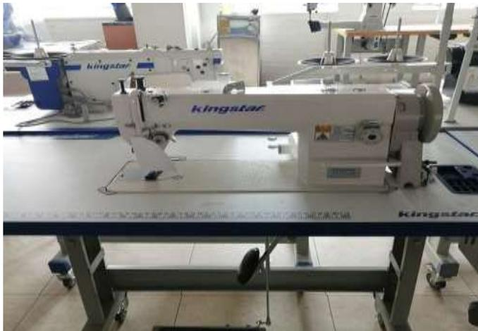
Industrial Walking foot machine: SABS approved or equivalent to Singer, metal/ wooden top only. Suitable for sewing light, normal/medium and heavy textile fabrics.
