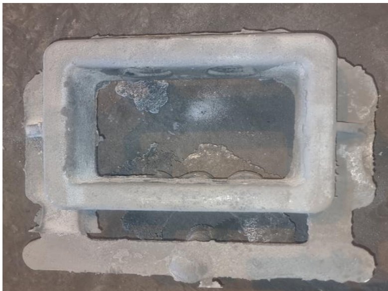
Figure 2: Bottom view of Coupler guides, as received by supplier.
