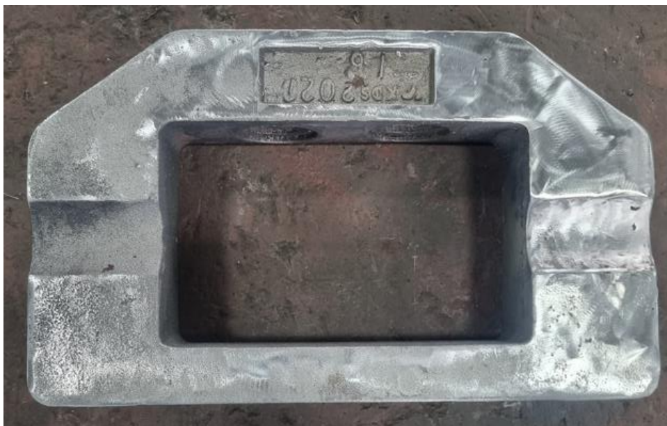
Figure 9: Illustrates the top view of a Coupler guide casting post grinding and dressing.
