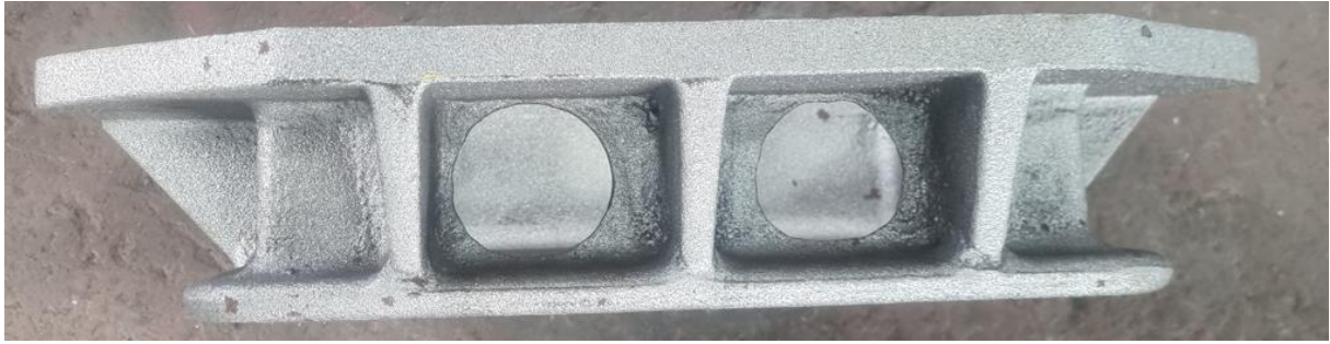
Figure 7: Illustrates the side view of a Coupler guide casting post grinding and dressing.
