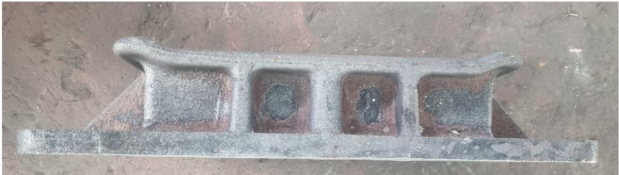
Figure 8: Illustrates the side view of a Coupler guide casting post grinding and dressing.
