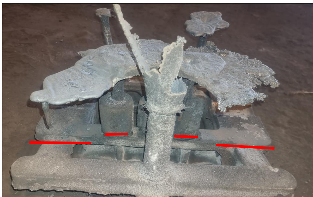
Figure 4: Illustrates the top view of the Coupler guides sections to be cut off by supplier.
