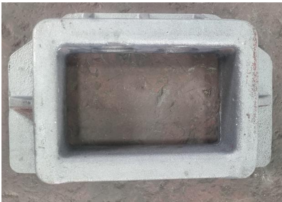
Figure 6: Illustrates the bottom view of a Coupler guide casting post grinding and dressing.
