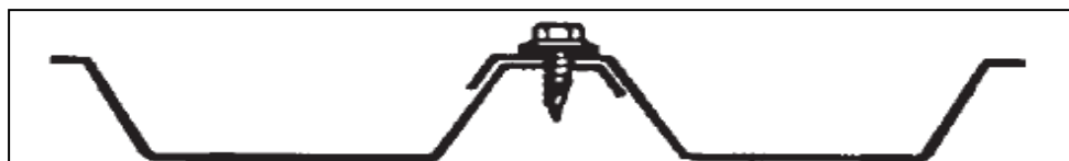
Figure 4 Typical side lap fastener details
