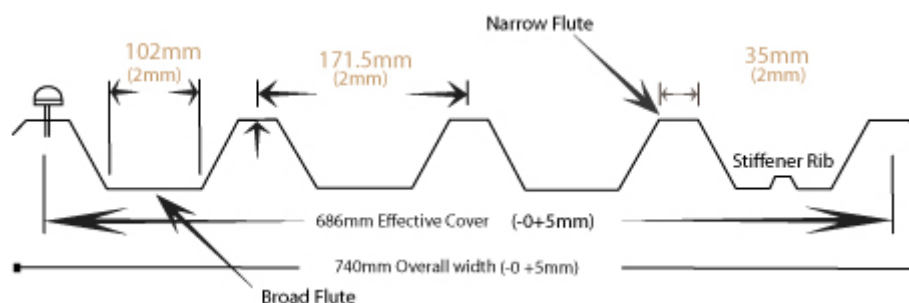
Figure 1 IBR 686 profile 0.54 mm
