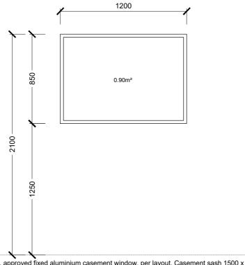
Type. D Crealco Swift 38 or eq. approved fixed aluminium casement window, per layout. Casement sash 1500 x 1200mm max capacity
