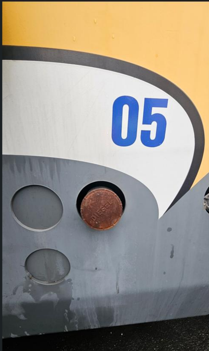
Reach Stacker - Filling Point with Cover (Wiggins Nozzle Used).jpg
