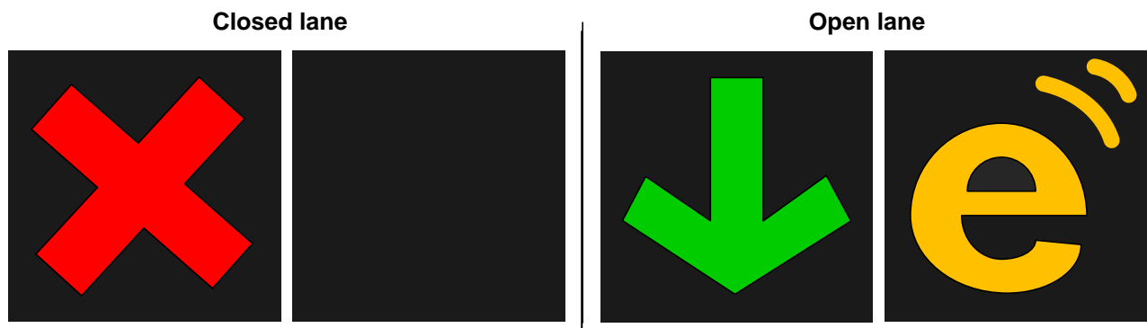
Figure 8-14: Typical OHLS configuration for a closed and open mixed ETC lane
