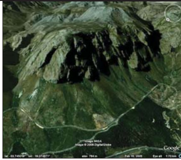
Du Toits Kloof Pass, old N1 route. Recurring rockfalls & debris flows disrupted traffic
