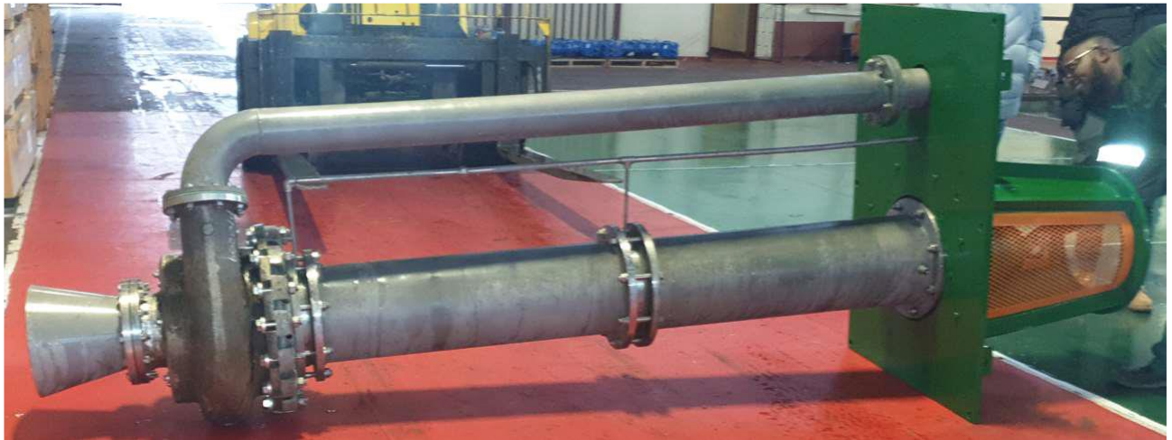
Fig.1: Tutuka P/S – Vertical Anion Supply Pump (3.0m length)
