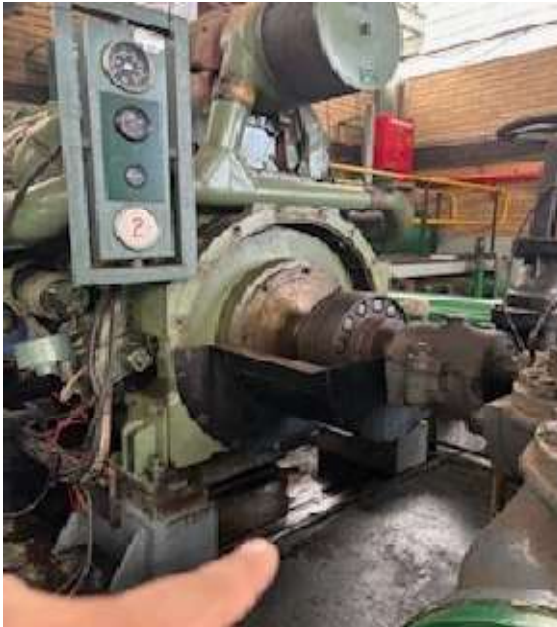
#2 ENGINE CRACKED SUMP
