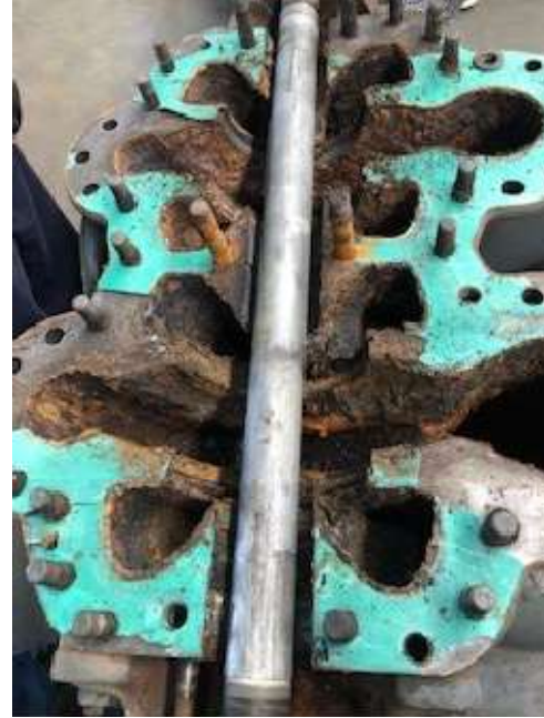
TYPICAL INSIDE OF PUMP BEFORE REFURB
