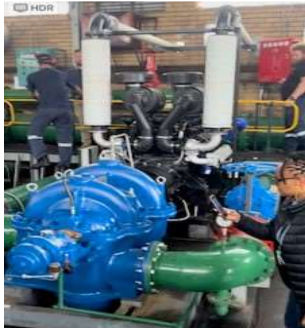
NEW ENGINE PUMPSET DELIVERING REQUIRED FLOW
