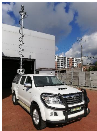
Figure 2.1: RFI monitoring vehicle
