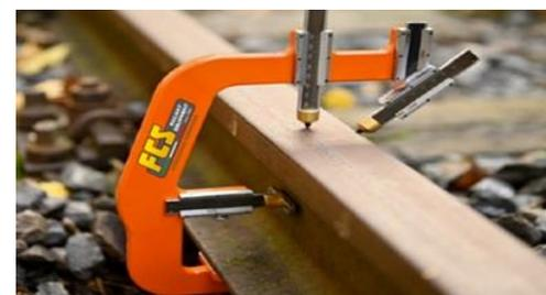
height dimension of the rail parallel to the base of rail on different rail types and lateral wear value at 45 degrees. The device can be easily attached to the rail base surface and fixes itself with six magnets built into its sole part and the side touch is ensured by a stopper.
