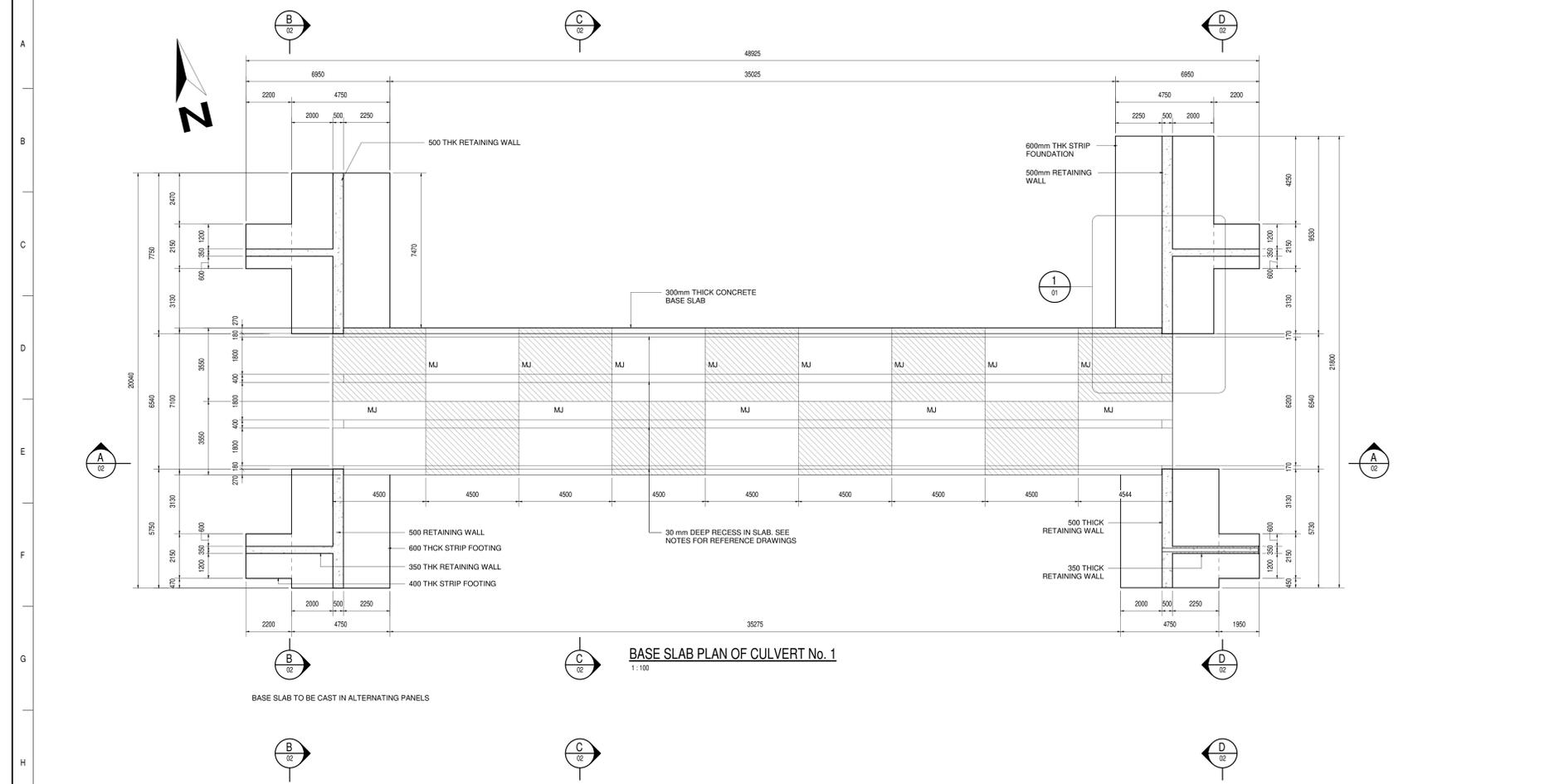
**BASE SLAB PLAN OF CULVERT No. 1**
