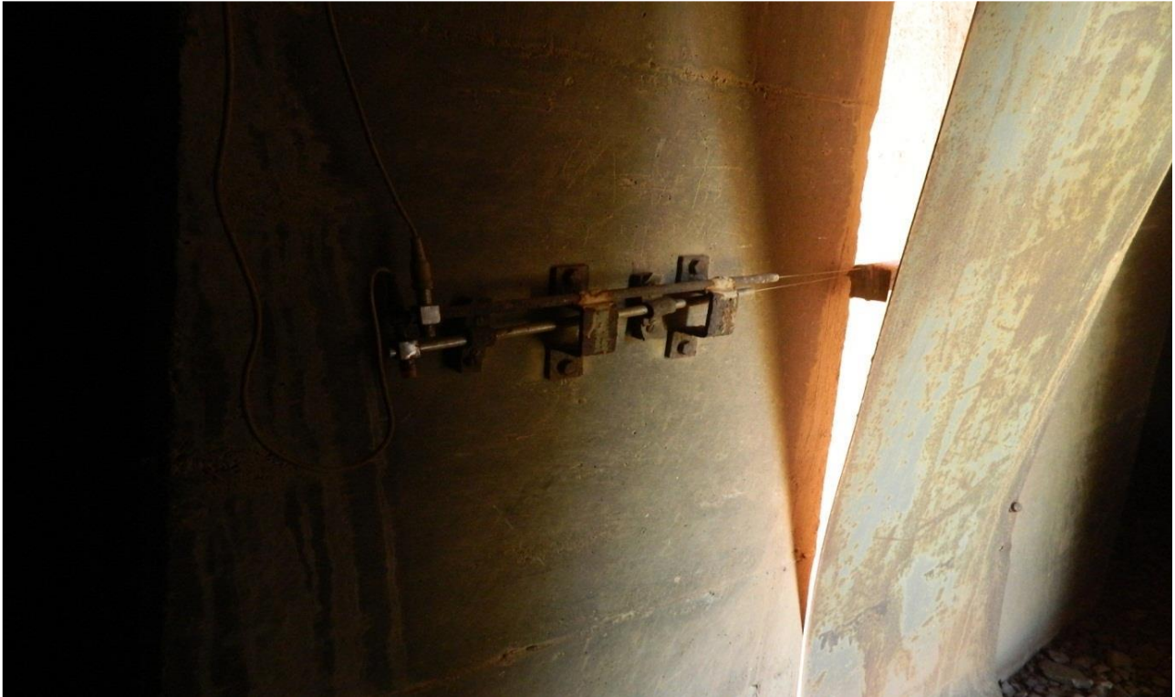
Appendix B Figure 18: Concrete deck deflection measurements sensors on the left hand side of the bridge deck at expansion joint 1 for system 1 and 2
