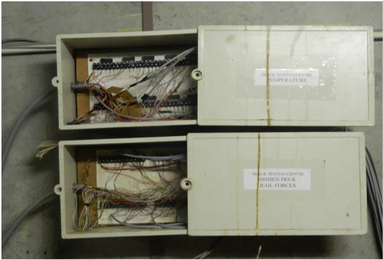
Appendix B Figure 20: Typical connections inside the interface box connection for system 1
