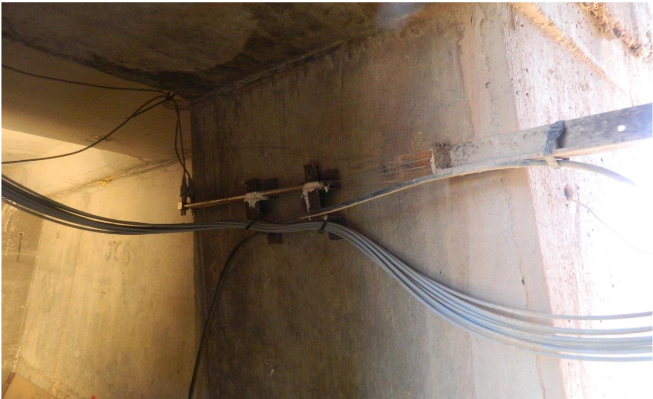
Appendix B Figure 16: Concrete deck deflection measurements sensors on the left hand side of the bridge deck at expansion joint 1 for system 1 and 2
