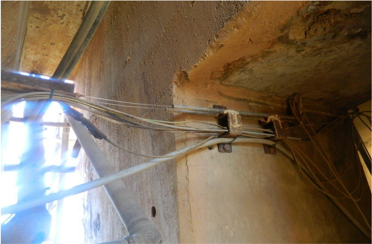
Appendix B Figure 15: Concrete deck deflection measurements sensors on the right hand side of the bridge deck at expansion joint 1 deck for system 1 and 2
