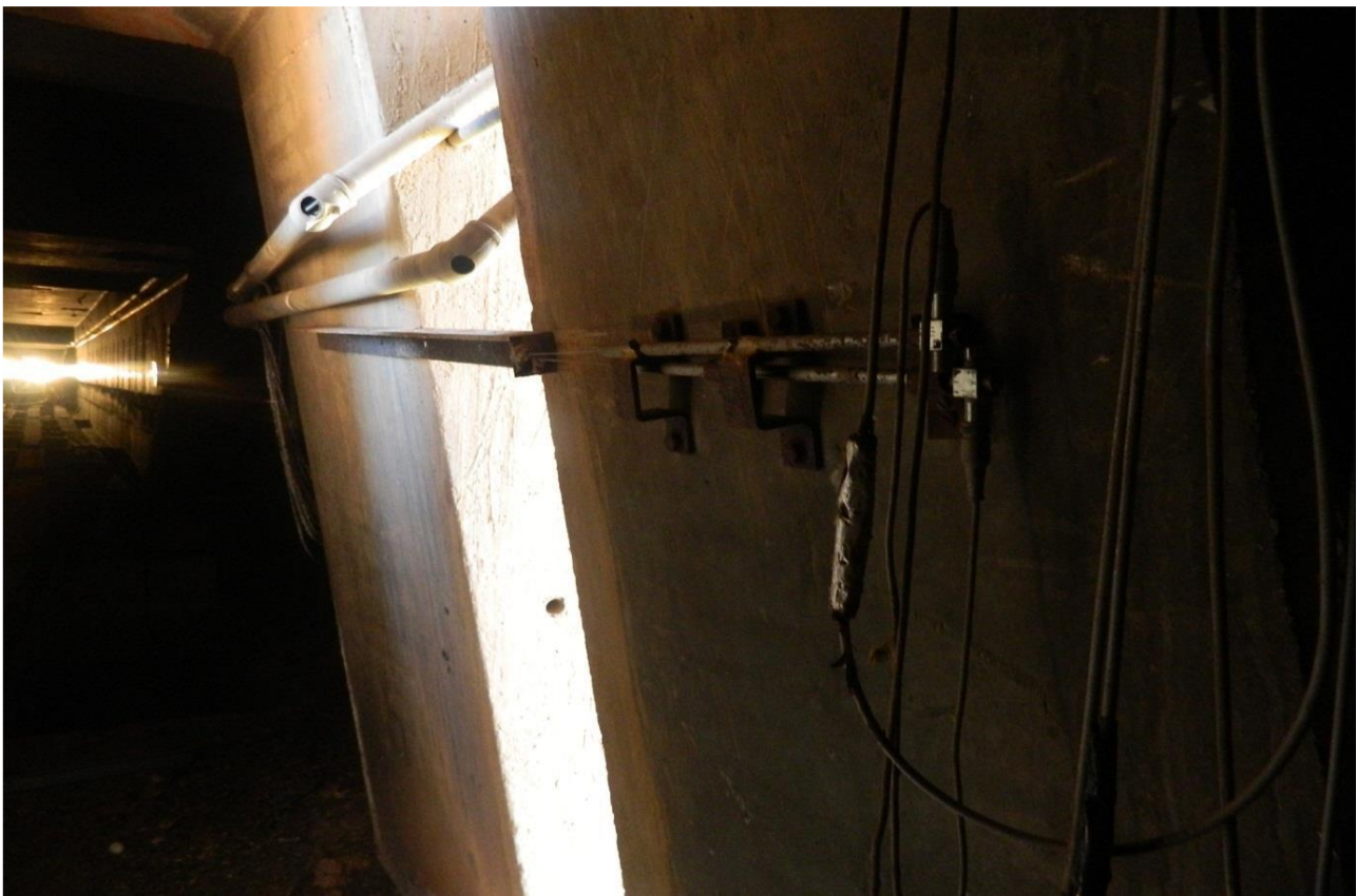
Appendix B Figure 17: Concrete deck deflection measurements sensors on the right hand side of the bridge deck at expansion joint 1 for system 1 and 2
