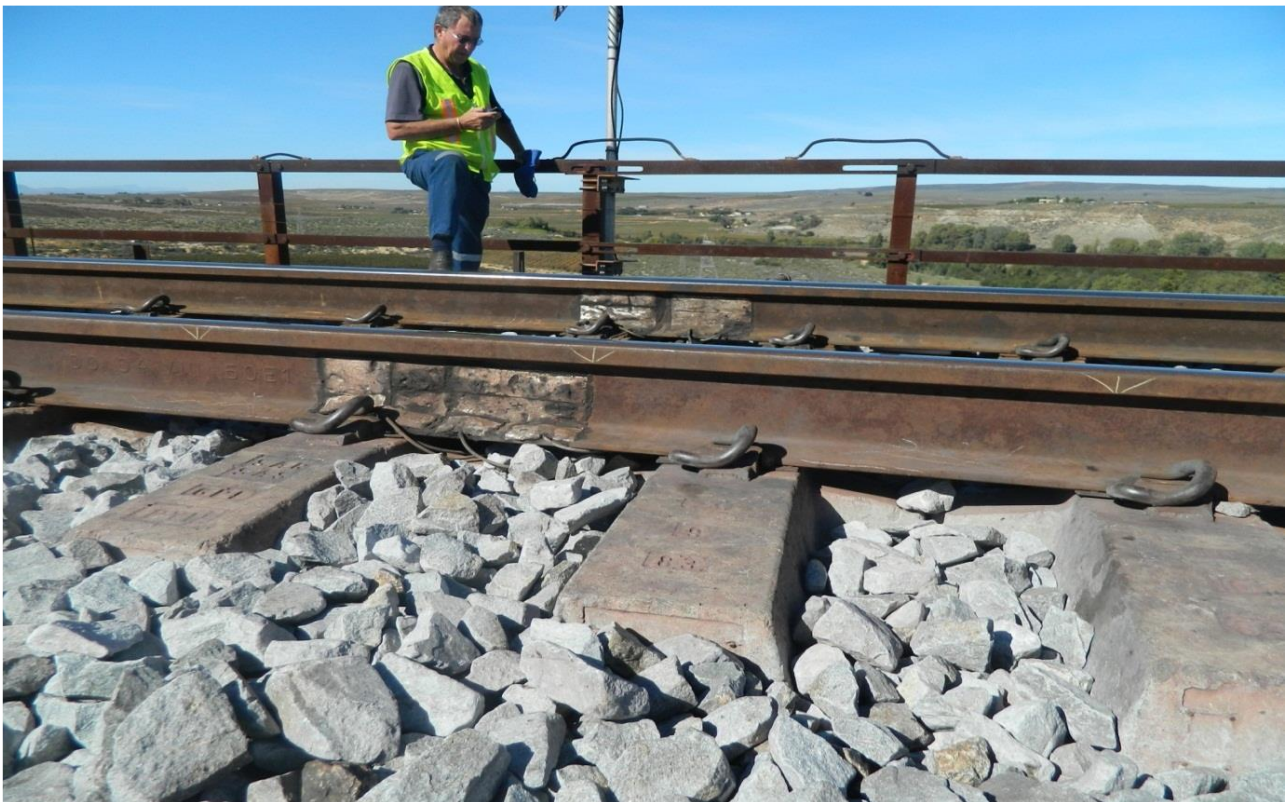
Appendix B Figure 9: Rail stress and temperature measurements sensors at expansion joint 1 for system 1 and 2
