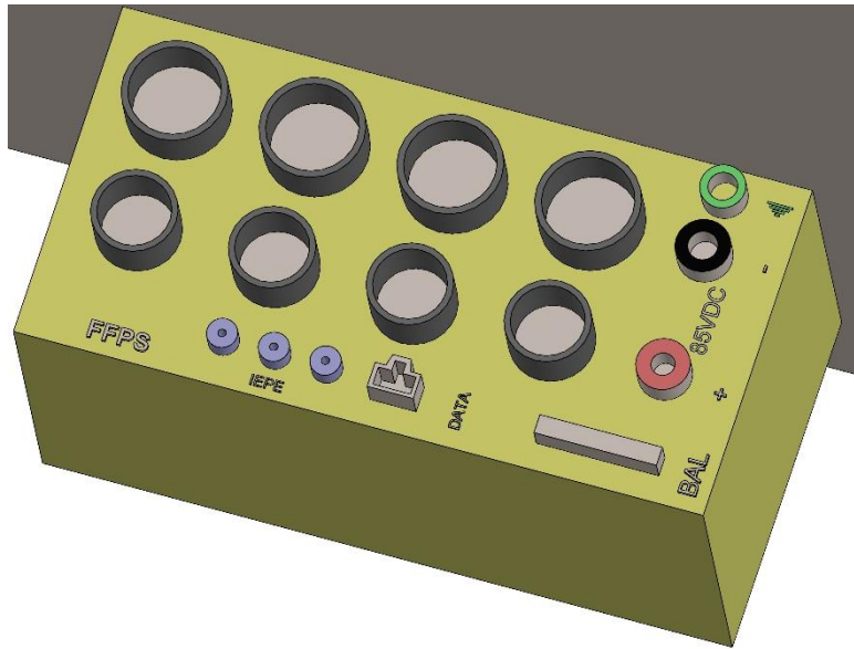
Figure 1-7 FFPS Junction Box model with plug receptacles
