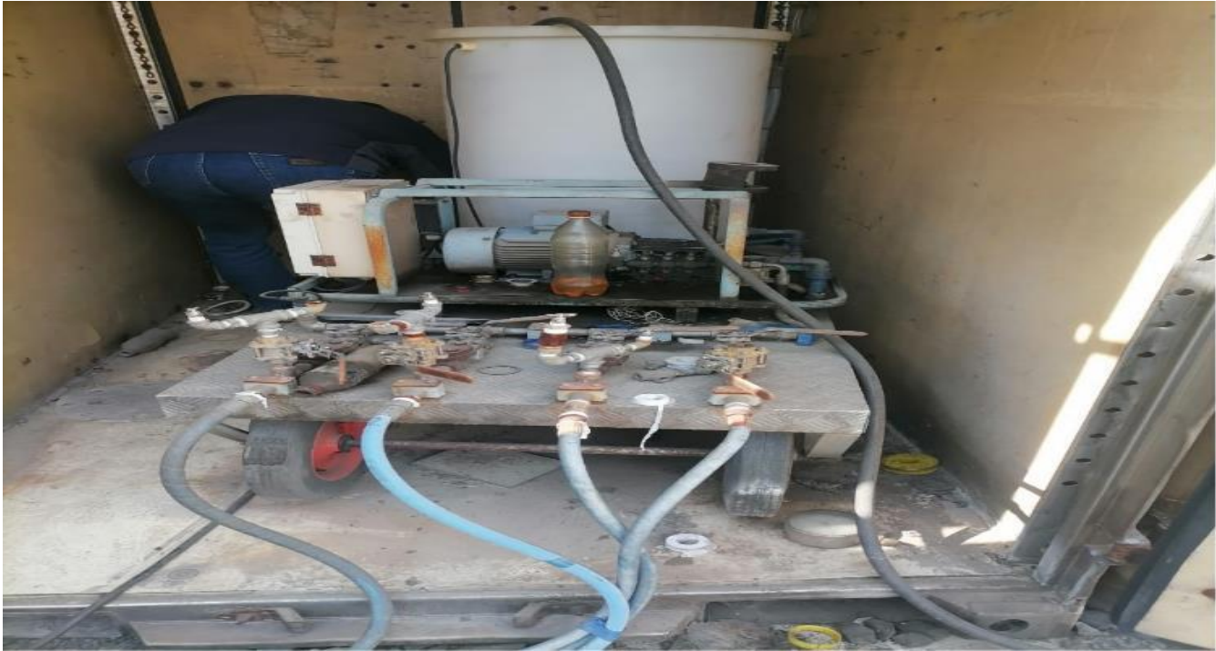
Trolley mounted pressure pump (B TEST)
