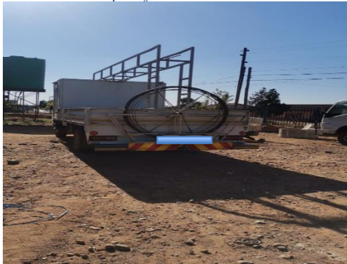
Picture 2: Example of Plumbers truck with mounted sewer rodding mechanism
